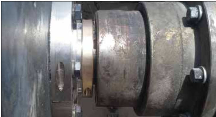
A split custom engineered Inpro/Seal Bearing Isolator provides permanent bearing protection on a Sag Mill Gearbox at a copper mine in the Southwest United States.
